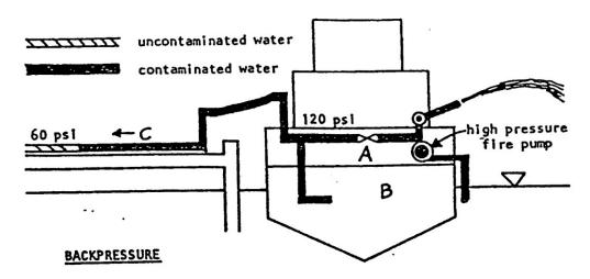
Example: Only the valve at A separates the potable and the sea water systems aboard a vessel. The vessel's potable water system, at B, is being filled from the public water supply system at C which is delivering water at a pressure of 60 psi. At the same time, the sea water fire fighting system is activated, which provides sea water at a pressure of 120 psi. If valve A is open, or leaks, the sea water will be forced into the public water supply system.
