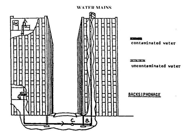
Example: A hose is submerged in a laboratory sink at A. Both buildings are connected to the same public water supply system, C. This main often lacks adequate pressure. The building on the right has installed a booster pump in the basement at B, in order to alleviate low pressures. The booster pump could deplete the water in main C, thereby subjecting the customer's water system to a pressure less than atmospheric thus causing a reversal of flow from the laboratory in the opposite building.
